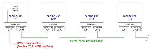
Each controller includes RS485 connector for easy BMS communication via ModBus RTU (a protocol allowing both continuously reliable and accurate remote control of the air-conditioning units) and a port for SNMP card (pCO Web).
