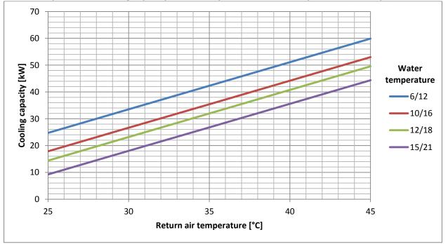
Conditions: maximal opening of 3-way valve.
