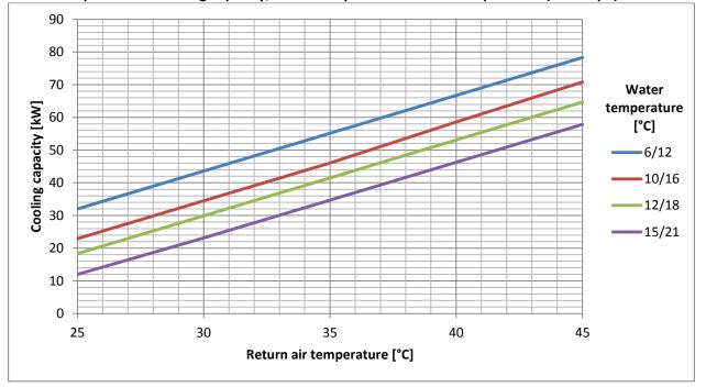
Conditions: maximal opening of 3-way valve.
