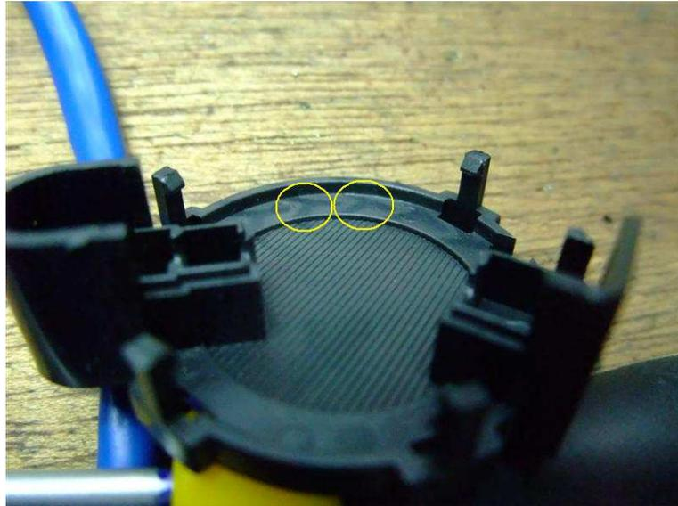
This picture above also shows the dust inside the cover of the Smoke Detector.
