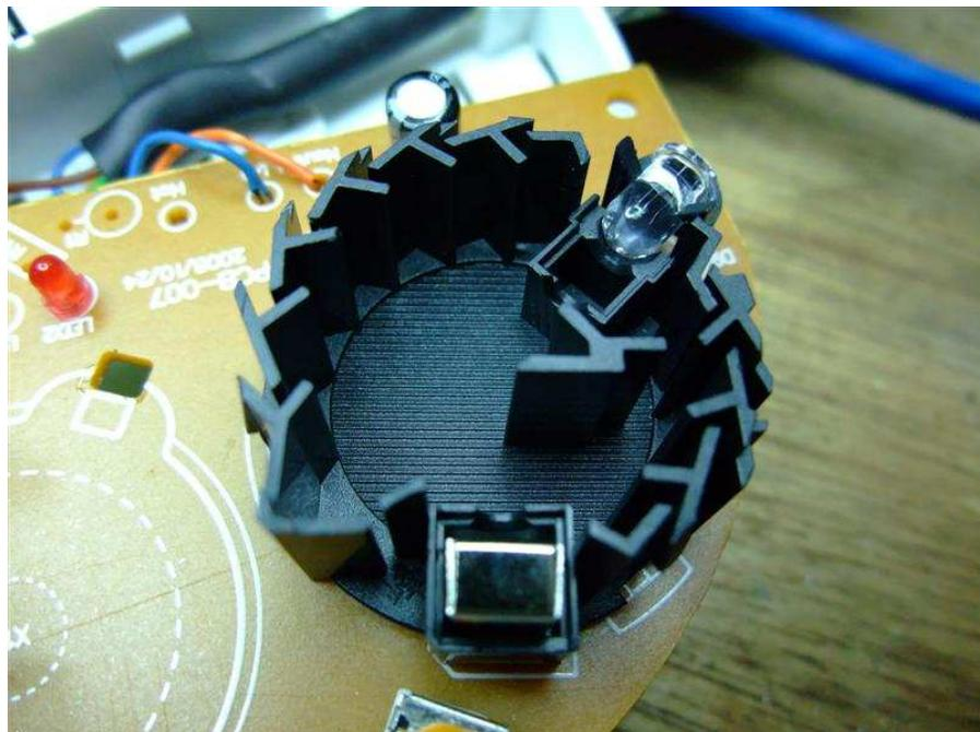
This picture above shows the optical chamber of the Smoke Detector after cleaning
