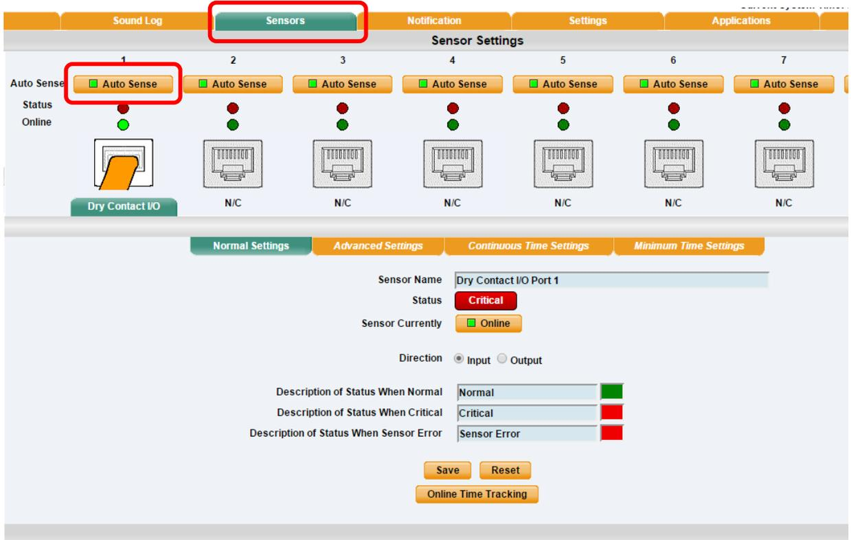
When you first connect the Smoke Detector to the RJ45 port it will be auto sensed online as a Dry contact I/O type sensor. Click the Auto Sense button as shown in the screen shot above.
