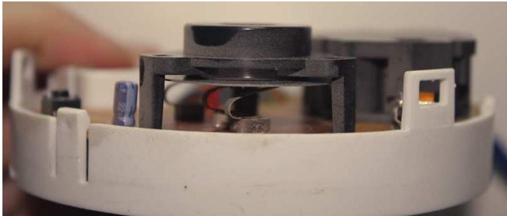
The picture above clearly shows the dust build up inside the detectors optical chamber. You can see the clear black plastic where we have wiped the dust off compared to the dusty surface.
